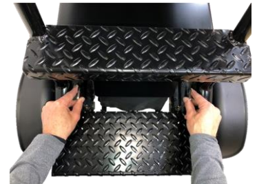
Freewheel feature allows rolling when powered down
