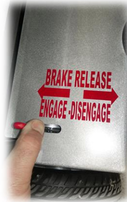
Freewheel feature allows rolling when powered down
